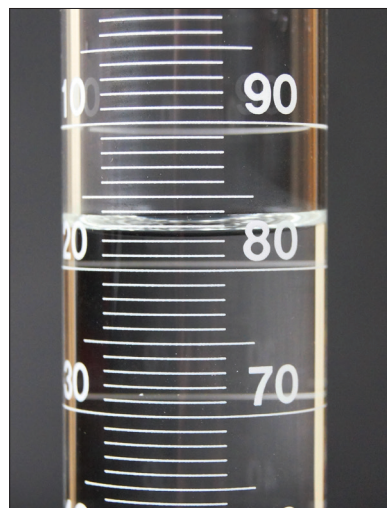
Figure 2.5. Reading the significant digits on a graduated cylinder.
