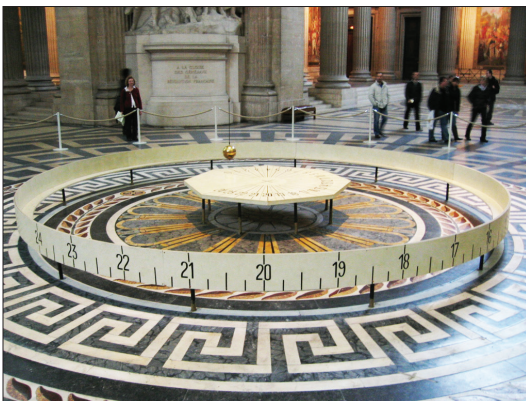
Figure 2.26. A Foucault Pendulum in the Panthéon in Paris.
