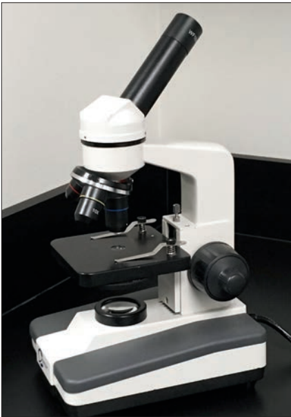
Figure 1.9. Compound light microscope. Instruments such as this provide magnifications of 40\text{--}1000\times .
