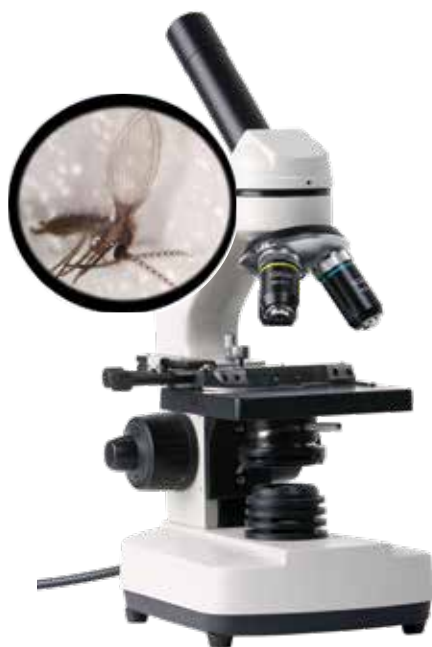
FIGURE 1.16 A Compound Light Micro- scope and Magnified Image of an Insect
